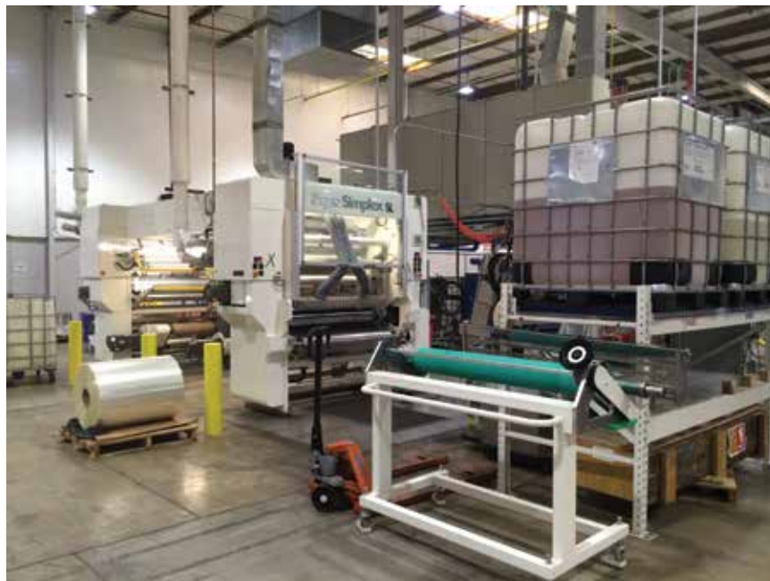
Poly Print has two laminators, one that's water-based and one that is solventless.
